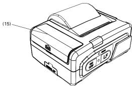
(15) Battery cover Cover of battery compartment
